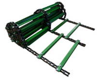
Feeder House Chains
