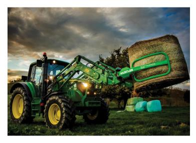
"Basically, the Softhands are used for handling silage bales without damaging the wrapping. Unlike other attachments, this Hustler product is hydraulic and offers a really gentle and precisely controlled grip on the bales."
